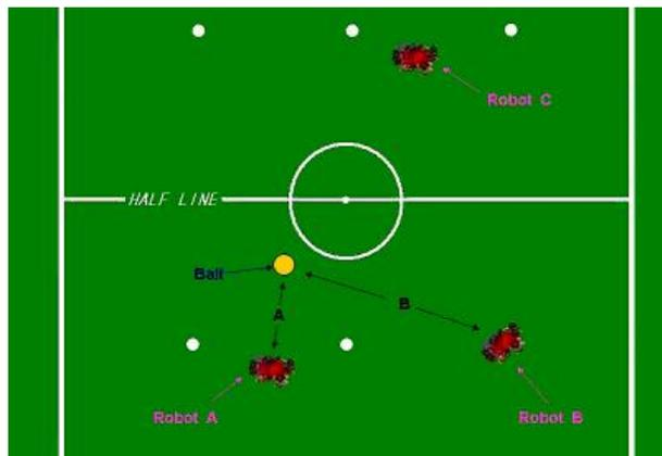
**Fig. 6.** Negotiation of roles for two robots based on distance from the ball and the strategy of the game.
