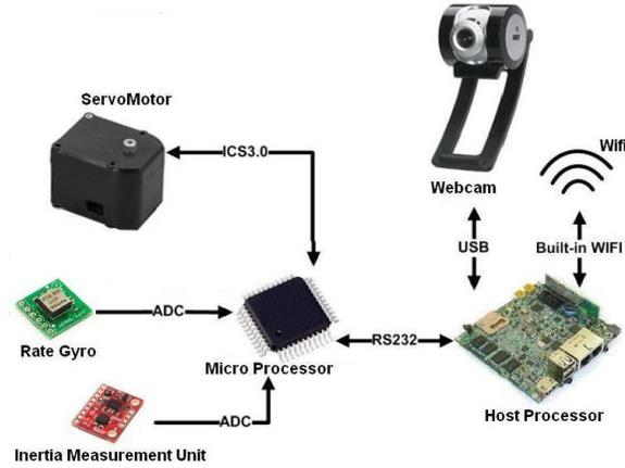
**Fig. 3.** Electrical system architecture
